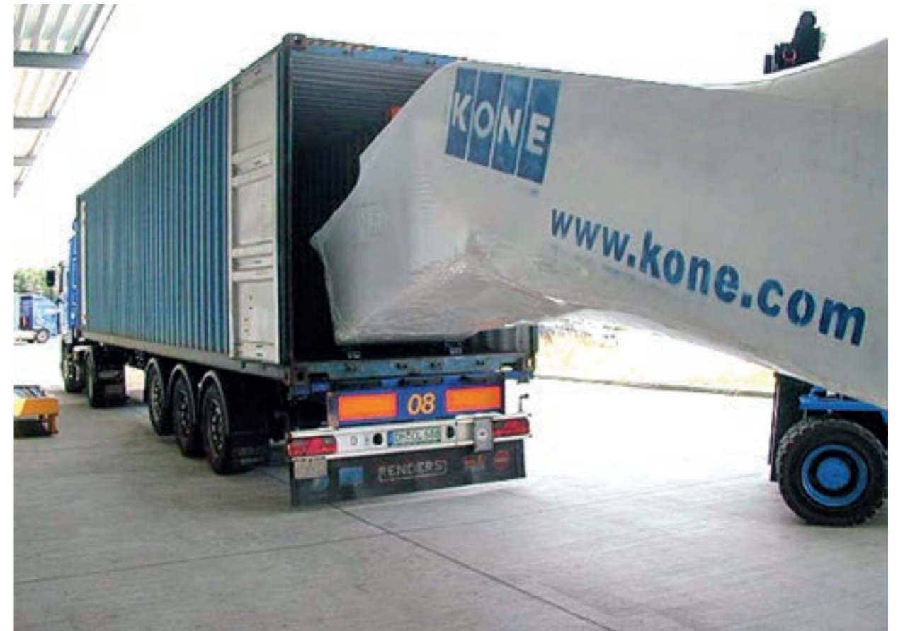
Figure 7.7 Unloading an escalator using forklift trucks
