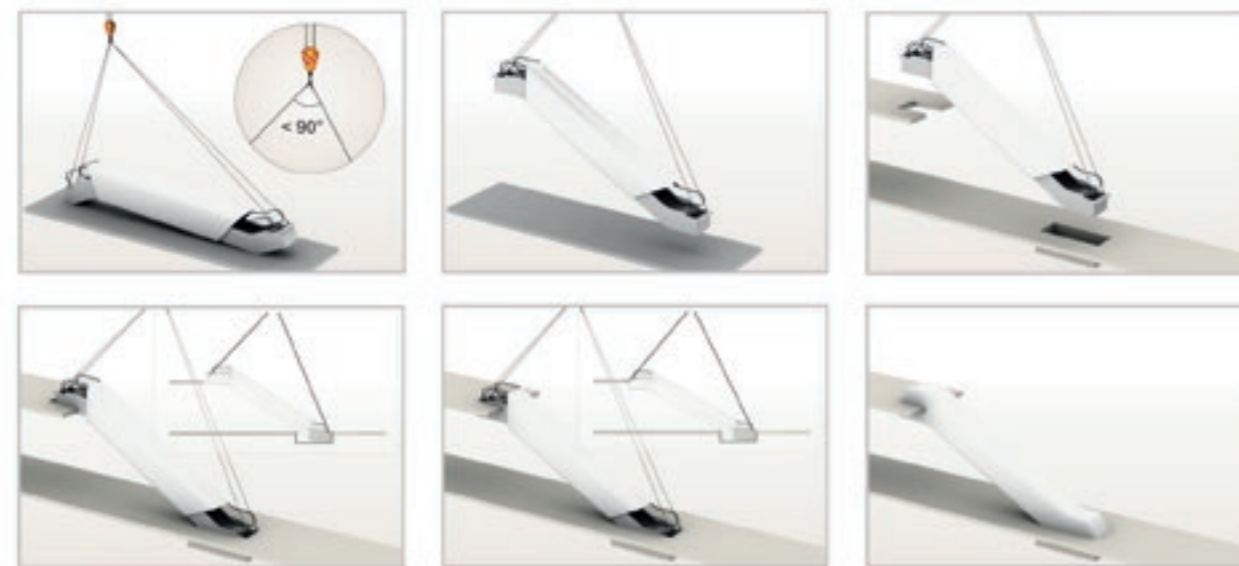
Figure 8.1 Installation in one complete section by a crane is probably the quickest and simplest method
