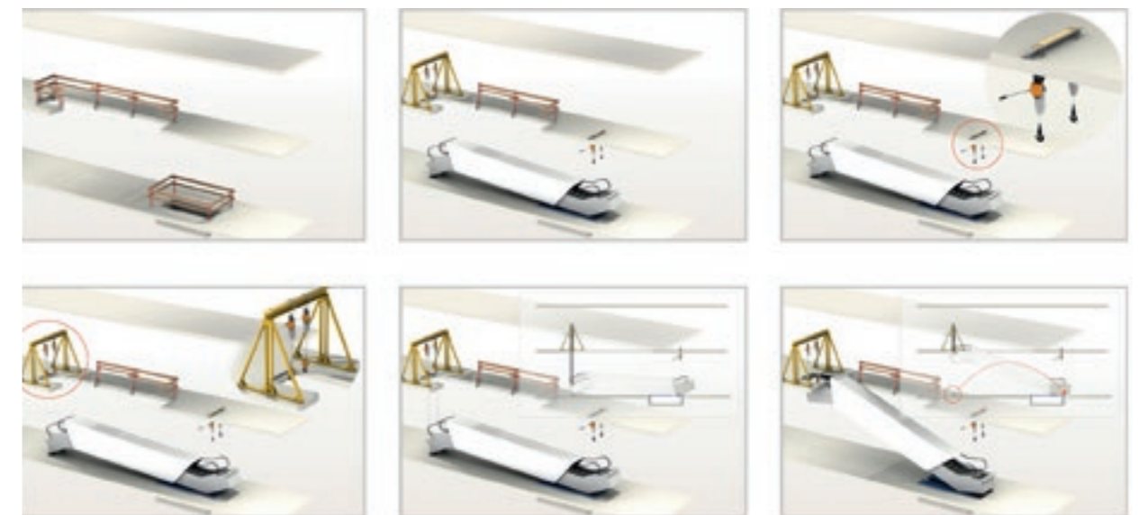
Figure 8.2 Installation in one section using A-frames
