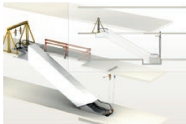
Figure 8.5 Installation using a lifting frame
