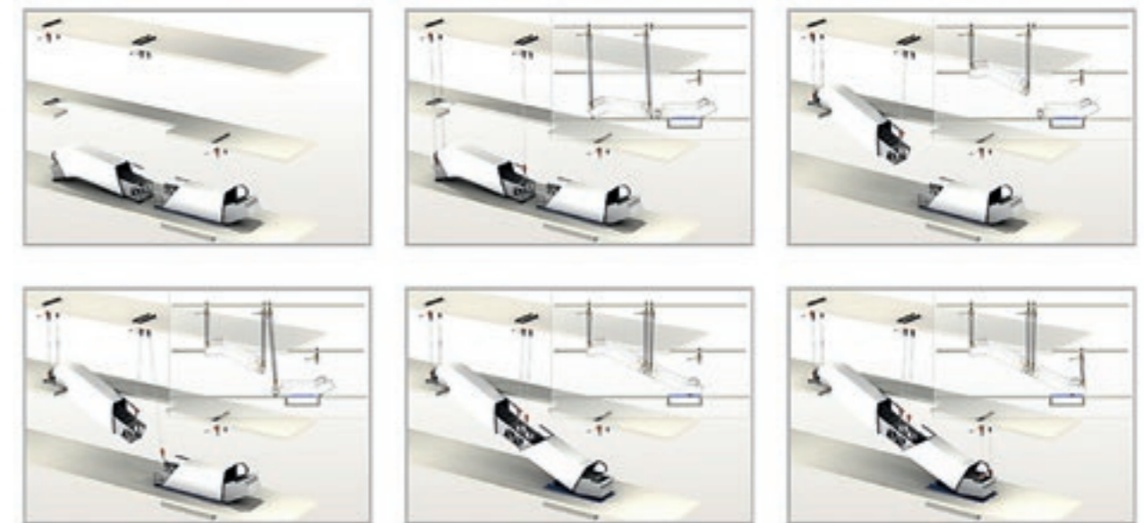
Figure 8.3 Installation in sections is useful when the roof of the building can not be removed
